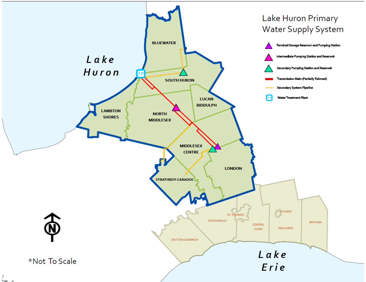
Figure 2: LHPWSS Major Infrastructure Locations
